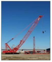
In November, the Port of Milwaukee received its brand new 300 Ton Manitowoc Model 2250 Crawler crane for use in the Operations Department. The new crane will primarily be used to load and unload breakbulk cargo for the Port's stevedores, Federal Marine Terminals. It's addition adds increased reliability
