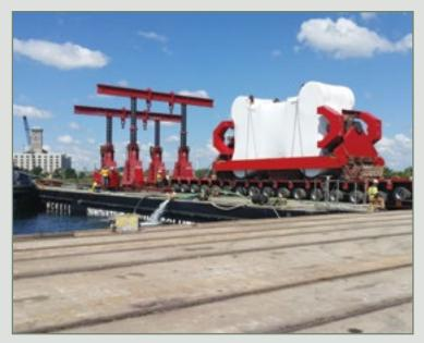
In September, Emmert International, a specialist in designing, engineering, and manufacturing heavy-haul and rigging equipment for project cargo movements, brought a 650,000 pound forge platen through the Port. It arrived on a McKeil Marine deck barge from the Port of Hamilton and was offloaded onto a Goldhoefer trailer at the Port's City Heavy Lift Dock on a sunny, calm Saturday morning.
